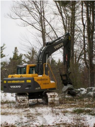
*An excavator-mounted mower clears trees to reclaim an old field on the Farrar Marsh WMA in Hillsborough.*
