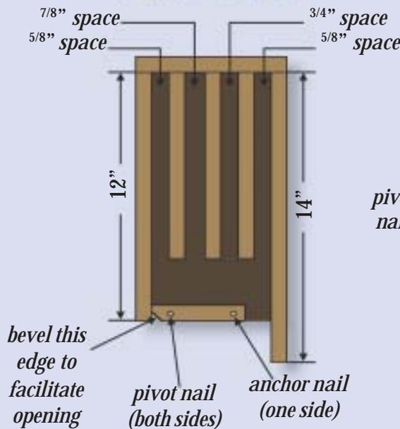
*Before assembling make sure you scratch up or roughen all interior surfaces. This will help the bats find some "grip" when entering and settling into the bat box.*
